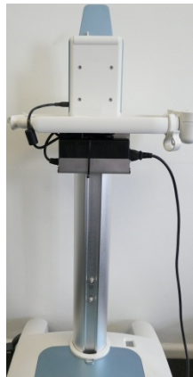
The Power Supply can be mounted in the dedicated bracket of the Roll Stand Basic
