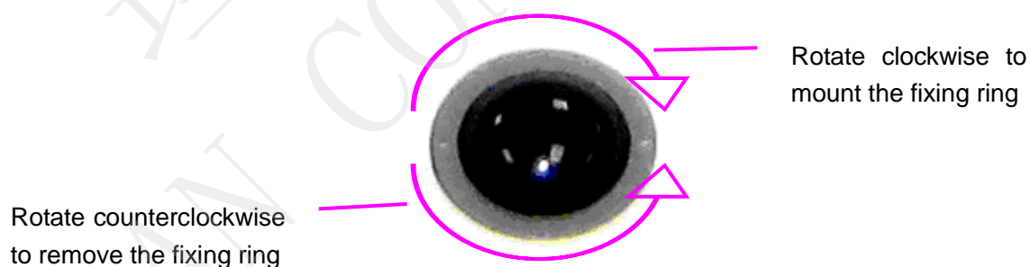
Figure 11-2 Assembling and Disassembling Trackball
