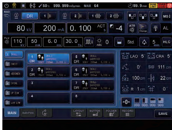
Anatomical programmed control (APC) for digital radiography (DR) setting
