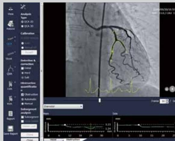
QCA\* features automatic contour detection and analysis of the area of interest. Various calibration options are available, such as Catheter, Sphere, and Distance calibration methods.
